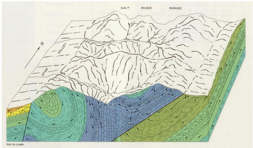
Generalized block diagram of part of the Salt River Range and Star Valley with arrows showing the inferred movement of ground water. Note the interbasin movement of ground water, the draining of rocks that overlie Paleozoic limestones or that have been butted against the limestones along thrust fault, and the concentration of flow through solution openings in the vicinity of spring.
